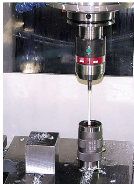
An example of a probe checking the dimensions. The shop produces the caps in conditions similar to those in a laboratory.
