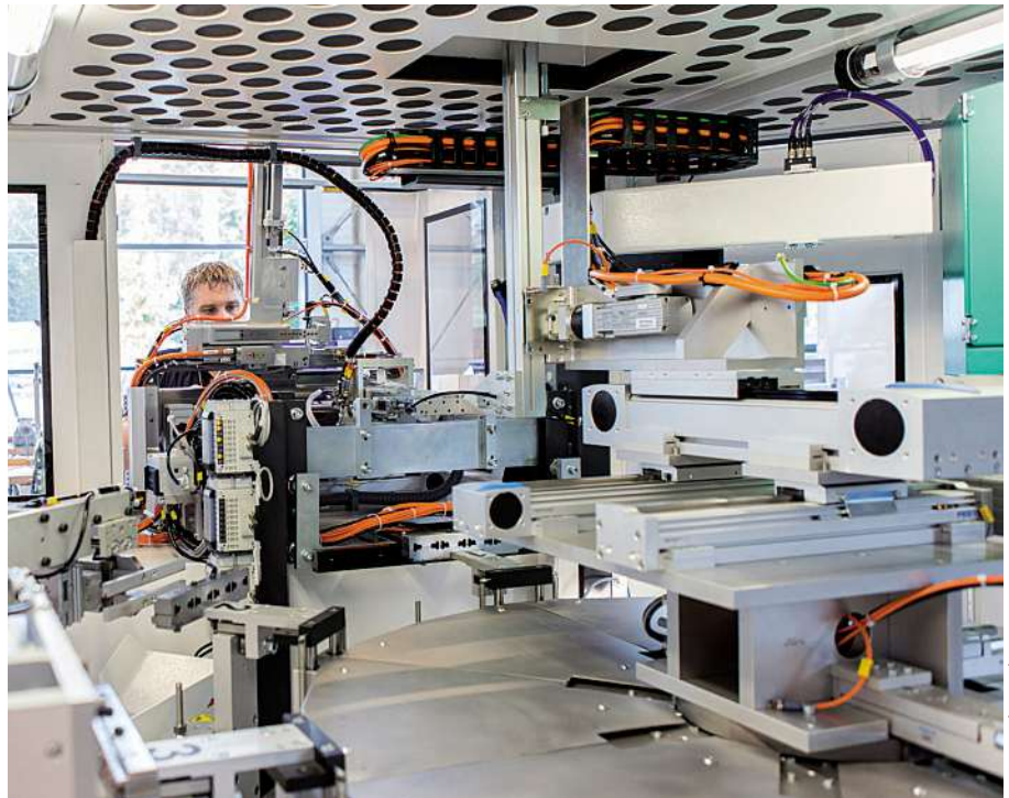
This system for making disposable syringes has eight stations and a high amount of throughput, according to tooling house Zahoransky.
